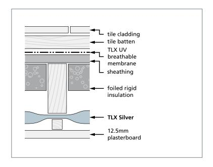
The cheeks of a dormer are generally of a new build timber frame construction. Timber studs give the strength to the wall, with sheathing board and breather membrane outside to ensure rigidity and water tightness. The outer cladding may be tiles, slates or weatherboarding.
