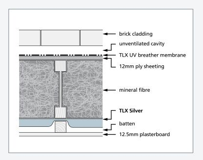
I-beam studs consist of two outer flanges held together by a thinner web. This introduces less timber bridging of the insulation between the studs and leads to lower U values. The flange is generally 39mm deep and 38-89mm wide and the web is 10mm wide. The total depth of the I-stud is 140, 200, 240, 300mm.
