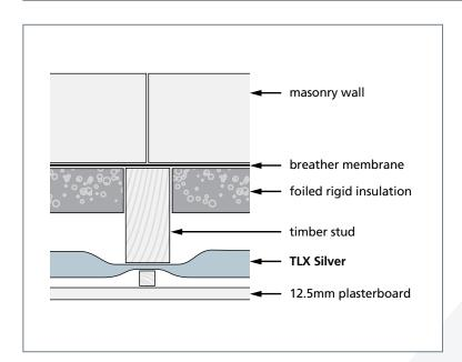
TLX Silver can be installed to the interior of cavity masonry walls, on timber studs or battens fixed to the inner leaf of the wall. A breathable membrane should be fitted between the inner leaf of the masonry and any timber studs or battens. Additional insulation may be fitted between the studs to lower the U value of the wall. A second set of battens holds the TLX Silver in place and provides a service cavity.
