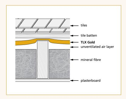
If the top 60mm of the rafter space is not filled with insulation, then TLX Gold can be laid across the rafters and allowed to drape down into the rafter space. Provided the TLX Gold forms a 10mm deep channel in the centre of the rafter space, then tile battens can be fitted directly on top of the TLX Gold without the need to counter batten.
