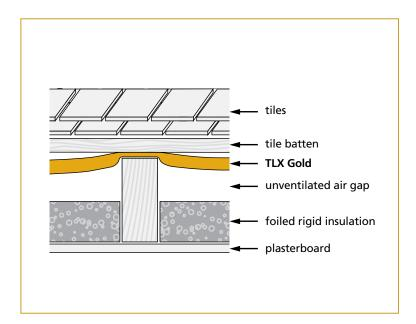
Where the roofline cannot be raised, it is possible to install TLX Gold draped over the rafters. TLX Gold will drape into the rafter by 50mm, taking into account a small unventilated air gap between the TLX Gold and additional insulation between the rafters.
