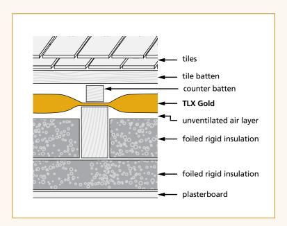
If there is scope to add additional insulation to the underside of the rafters as well as the between rafter insulation, this can further improve the thermal performance of the roof and will also limit thermal bridging.
