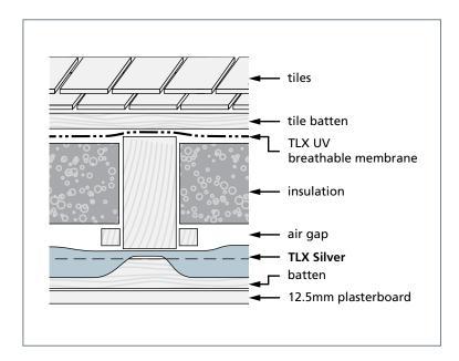
The rafters may need battening out to greater depth in order to accommodate the amount of insulation required. Rigid insulation board such as PIR or Phenolic board is fitted between the rafters. Boards can be held in place with small timber battens, clips or other fixings. TLX Silver is fitted across the bottom of the rafters, held in place with 38mm timber battens, and a sheet of plasterboard added.
