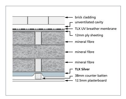
Split studs or twin frame is another way to reduce timber bridging of the insulation. The central layer of insulation is effectively unbridged by timber.
