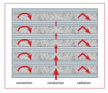
The outermost layers have low emissivity surfaces. These both reflect infrared radiation back into the house and prevent the house from emitting radiation to the outside. Inner layers of thick material such as wadding reduce heat loss by conduction through the multifoil, and inner layers of film prevent air movement. In addition, the insulation forms an airtight barrier reducing leakage of warm air to the outside.
