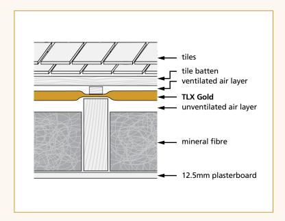
TLX Gold is a 2 in 1 insulating breather membrane, primarily designed to be used across the top of the rafters with additional insulation between the rafters. TLX Gold's top layer is a breathable membrane and so no additional roofing underlay is required. Additional insulation such as mineral wool is fitted between the rafters with an air cavity of around 20mm maintained between the mineral wool and the TLX Gold. Plasterboard can then be fixed directly to the underside of the rafters.
