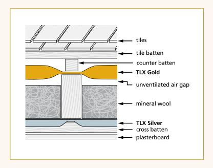
TLX Gold and TLX Silver can be combined when you have access from both the outside and inside of the building. TLX Gold is installed taut and counter battened over the top of the rafters. The additional mineral wool insulation is fitted between the rafters. TLX Silver is then fitted to the underside of the rafters secured by 38mm deep battens fitted crosswise then followed by the plasterboard.
