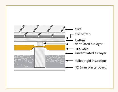
Where the roofline can be raised slightly, it is possible to install TLX Gold taut above the rafters, leaving enough rafter space for additional insulation. TLX Gold must be counter battened with minimum 38mm deep battens before the tile battens are fitted to create the channel required for air and water movement.
