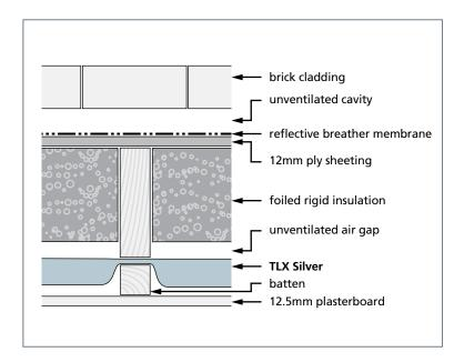
The thickness of rigid board is 20mm less than the stud depth, allowing an unventilated air cavity to form between the board and TLX Silver inside the studs.
