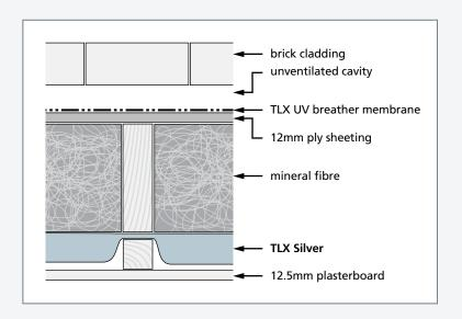
Fully fill stud cavity with mineral wool to prevent slumping.
