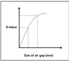
To achieve the optimal thermal performance with thin reflective insulation, it is important to provide small unventilated (still) air gaps adjacent to the reflective low emissivity surfaces. The air gaps should ideally be 20mm to achieve the optimal performance, taking into account the compression and expansion of the thin reflective insulation material.
