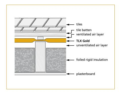
TLX Gold is a 2 in 1 insulating breather membrane primarily designed to be used across the top of the rafters with additional insulation between the rafters. TLX Gold's top layer is a breathable membrane and so no additional roofing underlay is required. Rigid insulation board such as PIR or Phenolic board is fitted between the rafters, maintaining an air cavity of 20mm minimum between the board and the TLX Gold. Plasterboard can then be fixed directly to the underside of the rafters.
