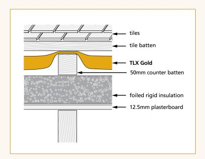
Plasterboard is first fitted above the rafters with a rigid insulation board such as PIR or Phenolic board fitted above it. A 50mm deep counter batten is then fitted above the rigid insulation board maintaining an air cavity of 10mm minimum between the board and the TLX Gold.
