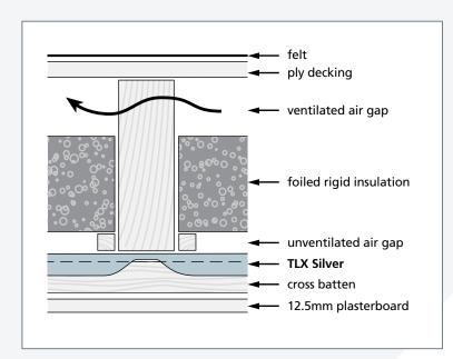
The most effective way to alter the U value is to vary the thickness of rigid insulation. However, maintaining the air cavities is critical and reducing the depth of any cavities to below 20mm to allow for more rigid insulation is unlikely to improve the U value.
