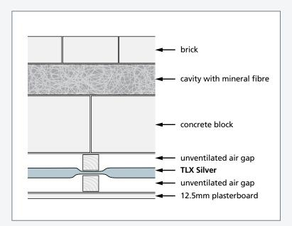
Masonry cavity walls are a traditional and widely used method of building walls. The cavity can be fully filled with insulation, either fitted or injected, or partially filled to leave a clear cavity.
