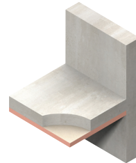
Insulation for structural ceilings (soffits)
